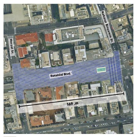
FIG. 4 Top view of the full-scale representation of the Azrieli Center façade on Rothschild boulevard [credits: the Authors]
