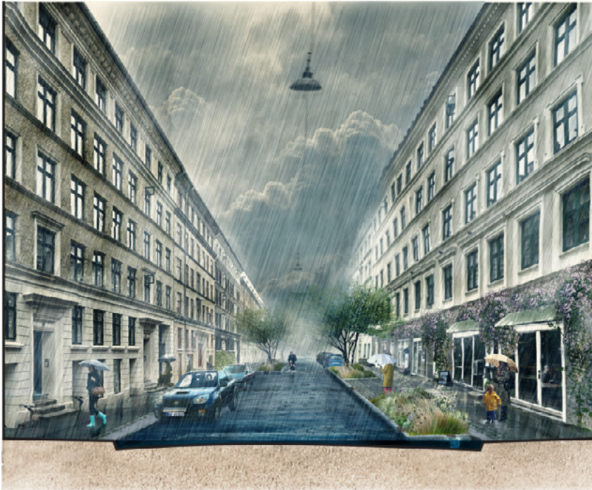
FIG. 13 Copenhagen, retention road, illustration from “Cloudburst typologies” developed by HOFOR, EnviDan and Urbanisten for the city of Copenhagen (2014)
