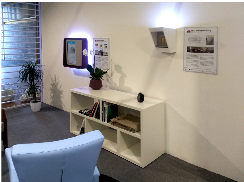
FIG. 5 The image shows the functioning prototypes of the HABITAT system: the digital 'frame' interface (top-left); smart chair; and indoor localization system inside the lamp (top-right). Source: M. Marchi, 2019
